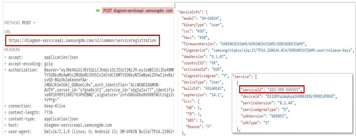
Fig. 6. A packet that registers the list of diagnostic data collection target apps managed by the “DiagMonAgent” app on the server.
